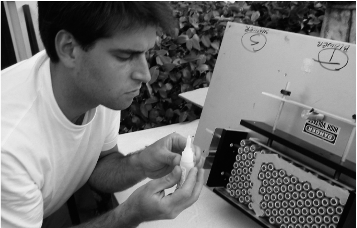
JB Straubel puts together one of Tesla Motors's early battery packs at his house. Photograph courtesy of Tesla Motors
