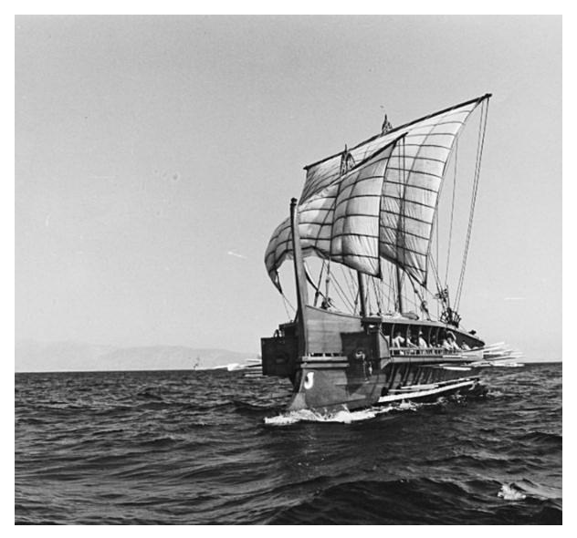
**Figure 9.2. The trireme** *Olympias.* This reconstruction of the most famous class of Greek warship, the trireme, was built and tested for seaworthiness in the 1980s in Athens. With a heavy bronze ram, a trireme was essentially a maneuverable ramming machine. Its light weight meant that a trained oar-crew could reach a speed of up to fifteen knots. © RMN-Grand Palais / Art Resource, NY.
